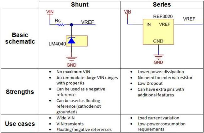
Table 1: Typical comparison table of shunt versus series voltage references
